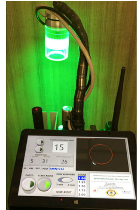
This instrument, which was invented at the Ophthalmic Biophysics Center with financial assistance from Florida Lions Eye Bank, emits green light for Photodynamic Antimicrobial Therapy.
