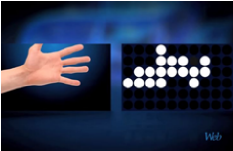
A graphic shows how basic the image of an outstretched hand appears to a patient using the Argus II device.
